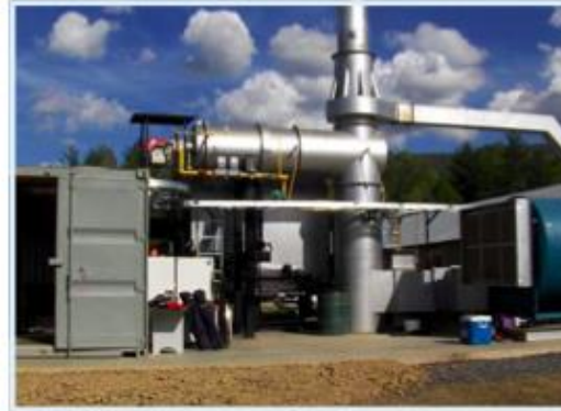
Gasifier disposing of manure and supplying thermal energy to poultry farm in West Virginia
