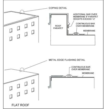
membrane (see detail figures) is an effective means of strengthening the attachment.
