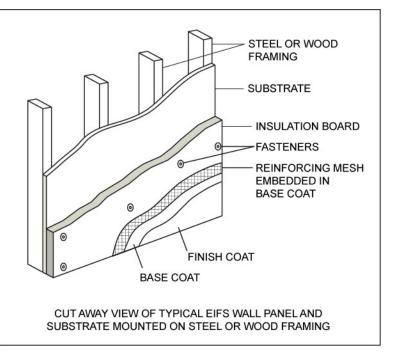
You should periodically inspect your EIFS walls, particularly the flashing where the walls meet the
