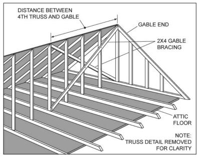
✓ The detail featured on this Fact Sheet provides increased resistance of the gable end to wind loads. For another gable end retrofit that meets current building code requirements, see FEMA P-804, Wind Retrofit Guide for Residential Buildings.
